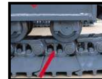
Track Link with Strut PC270-7 uses track links with strut providing superb durability
