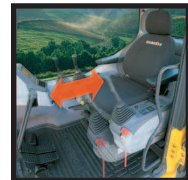
Seat Sliding Amount: 340 mm 13.4", increased 120 mm 4.7"
