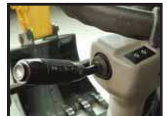
Tiltable steering wheel with several functions; wiper control, indicator, horn, and head lights Courtesy of MachineMarket
