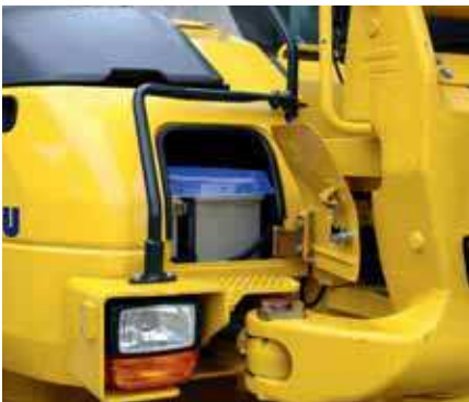
Ground level battery access
