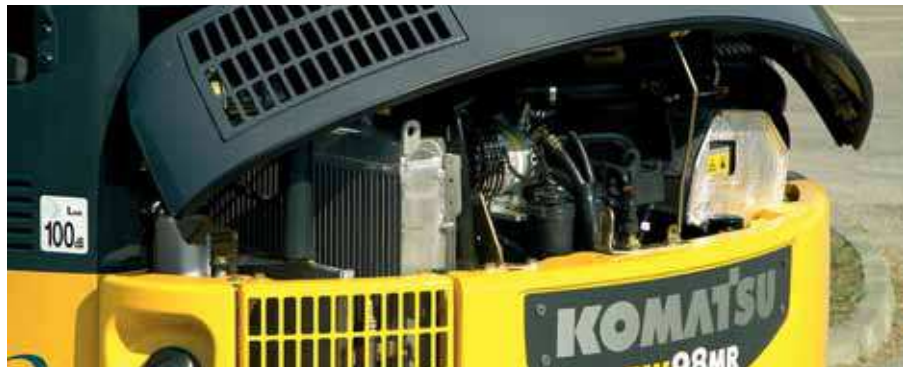
All periodic inspection points are easily accessible
