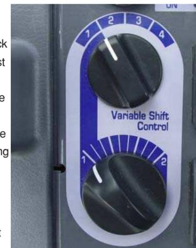
The variable shift switch allows the operator to adjust his machine speed in confined v-loading applications. When in 1, the operator can adjust his travel speed using the variable shift switch to match his machine speed and hydraulics to the distance he must travel.
