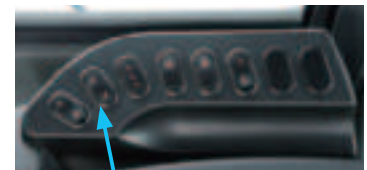
Dual mode engine power selection switch
