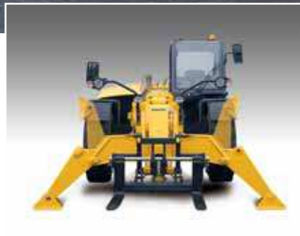
Wide type stabilisers guarantee highest stability on any ground type. Cylinders are well protected inside the frame.
