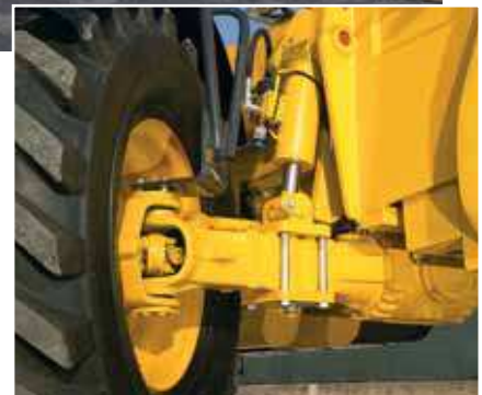
An optional automatic rear axle oscillation lock enlarges the bearing area, thus increasing both lift performance and security and reducing the risk of lateral tipping. It engages automatically over a 50° boom angle.
