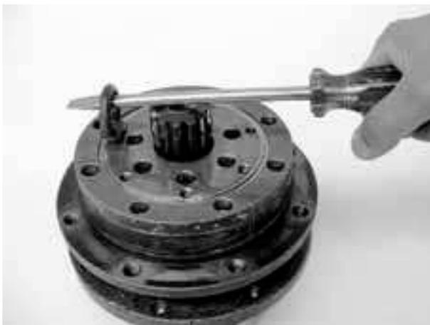
4) Fit an eye bolt to the valve plate (17), hook it on screwdriver and lift the valve plate (17) from the wheel (10)
