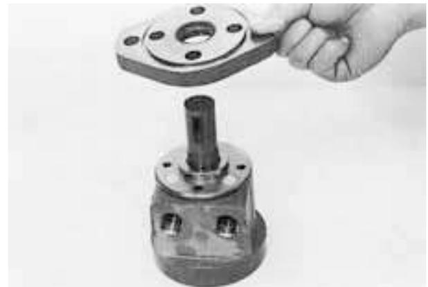
(9) Mount flange into housing saay. Care should be taken not to damage seal with shaft key.
