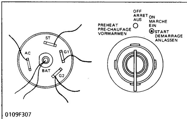
The key switch has 4 positions. The terminal "BAT" is connected to the battery.
