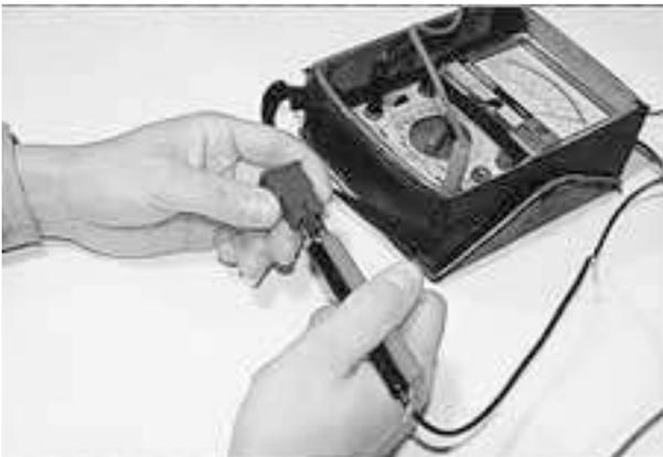
1. Checking slow-blow fuse for breakage (Photo 3)
