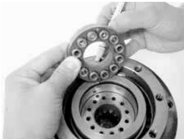
12) Fit the valve in the valve sleeve (7). Align the phase position so that pins are fitted in.
