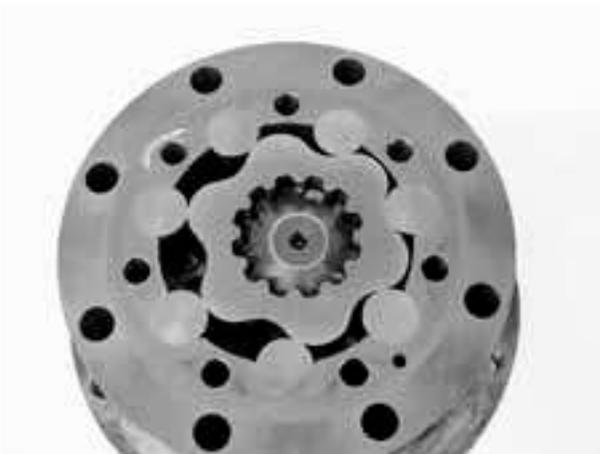
16) Mount the O-ring (26) onto the valve plate (17). Align the phase with one of the six crests of the star (2) and mount the geroller (4).
