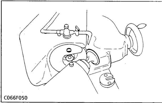
**Correcting Valve and Valve Seat**
