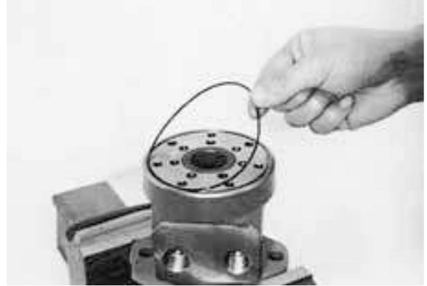
(11) Clamp with vise at flange and put O-ring on housing.
