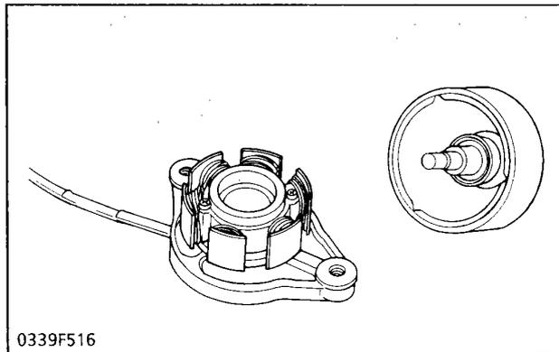
This dynamo is an 8-8 pole rotating magnet type generator. It is simple in construction, consisting of a stator and rotor. The rotor is made up of eight permanent magnet pole pieces assembled on a shaft and rotates on the center of the stator around which eight electromagnetic coils are provided. This dynamo produces higher voltage in slow speed rotation, and charges electric current to the battery during engine idling.
