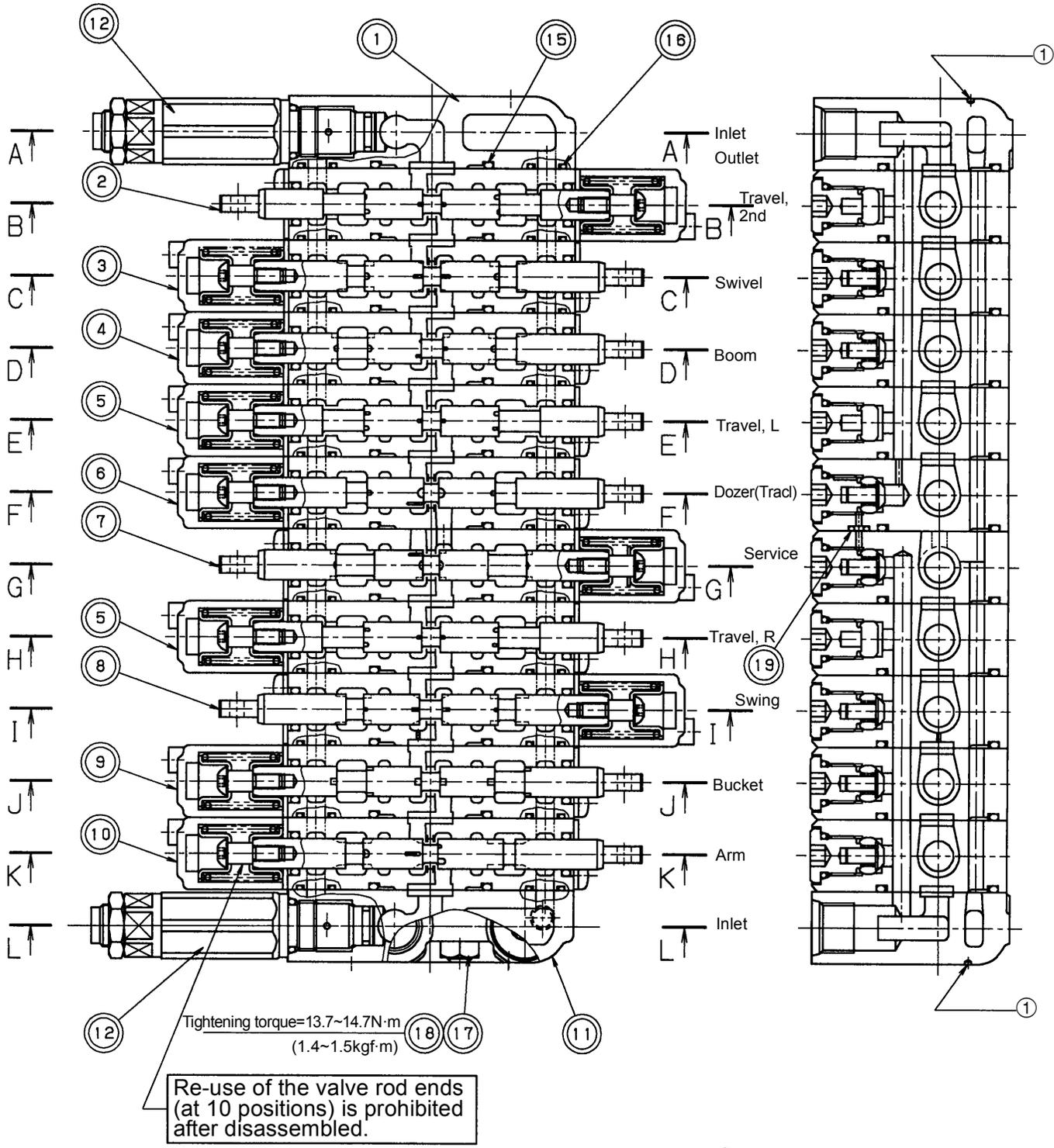
①Drilled hole for identification
