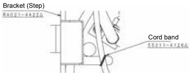
\* Clamp the cord band securely to the bracket (step).
