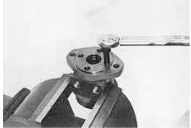
(11) Mount the motor housing by vise as shown in photo, remove 4 pieces of flange mounting bolts.
