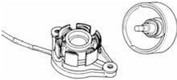
This AC dynamo is so designed as to mount a cooling fan at the shaft end and composed of a rotor and stator.
