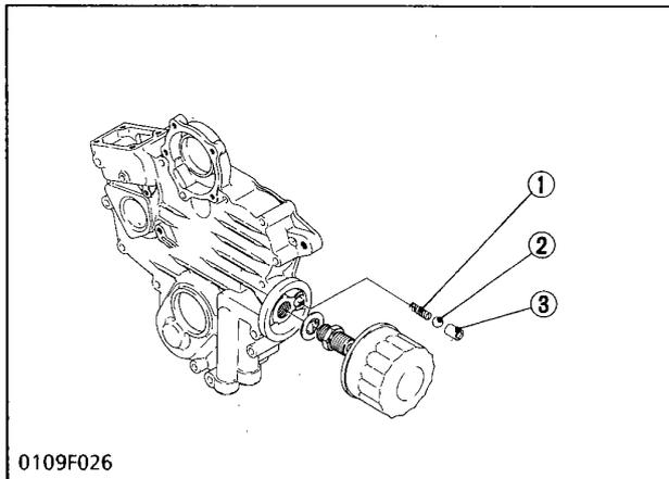
The relief valve prevents the damage to the lubricating system due to the high pressure of the oil.
