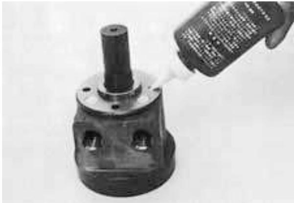
(8) Thoroughly clean flange mounting screw holes of housing, remove grease and apply screw-locktite slightly. (S-280 and S-380 dose not require this job.)
