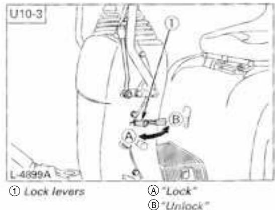
a. Control lever lock being at lock position
