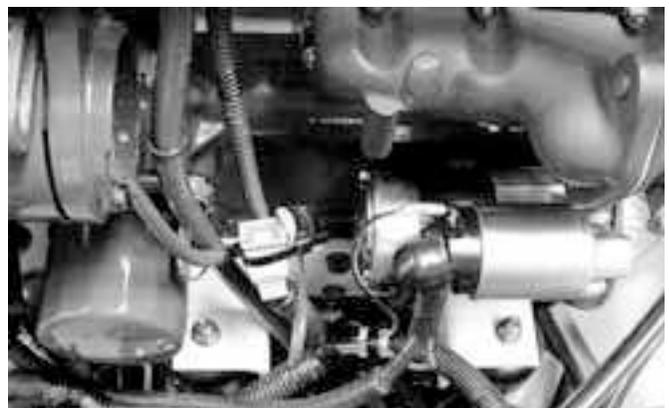
(G) Clamping of the battery plus cord and the wire harness (1) to the swivel frame.
