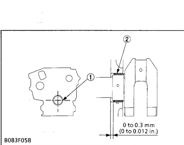
(1) Seam (2) Crankshaft Bearing 1
