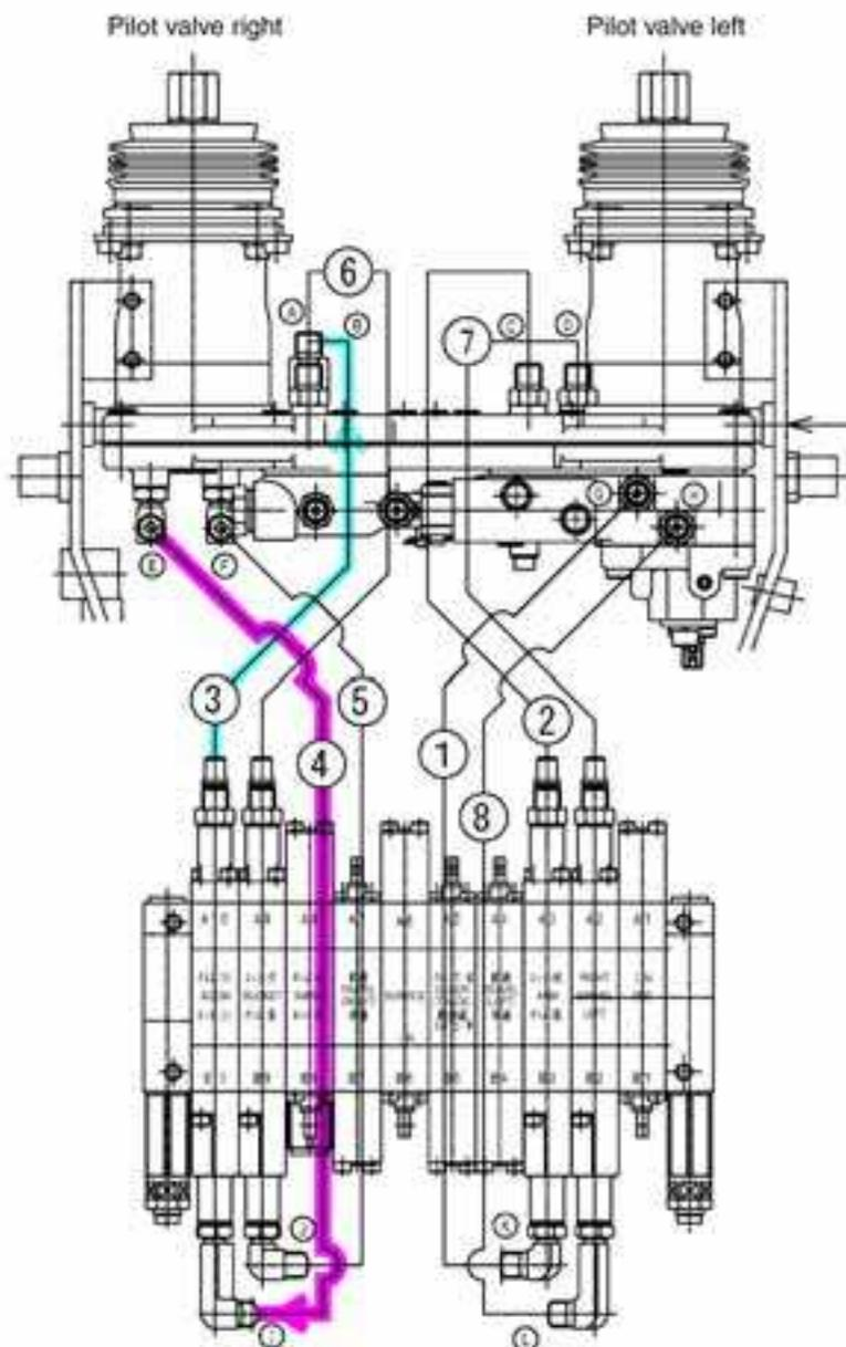
c. Flow of oil in boom lifting operation
