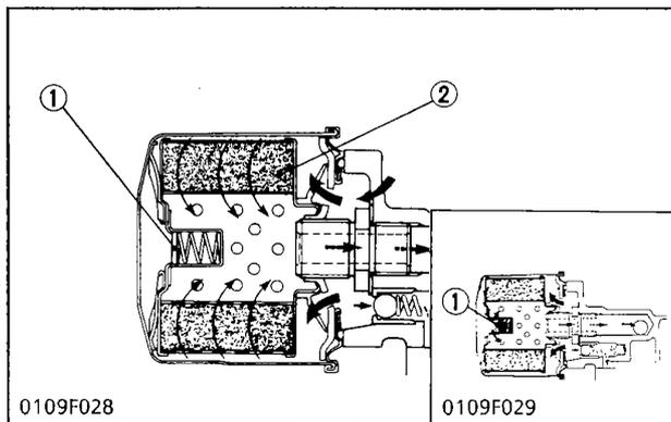
After lubricating, the lubricating oil brings back various particles of grit and dirt to the oil pan. Those particles and the impurities in the lubricating oil can cause wear or seizure of the engine parts. It may also impair the physical and chemical properties of the oil itself.
