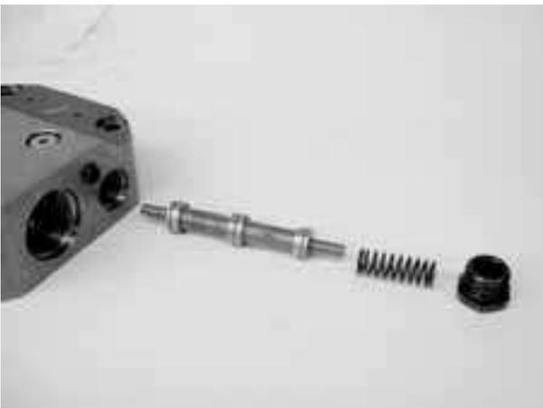
14) Remove the plug (V4), spring (V3) and spool (V2). (Do not use spanner but use socket wrench.)
