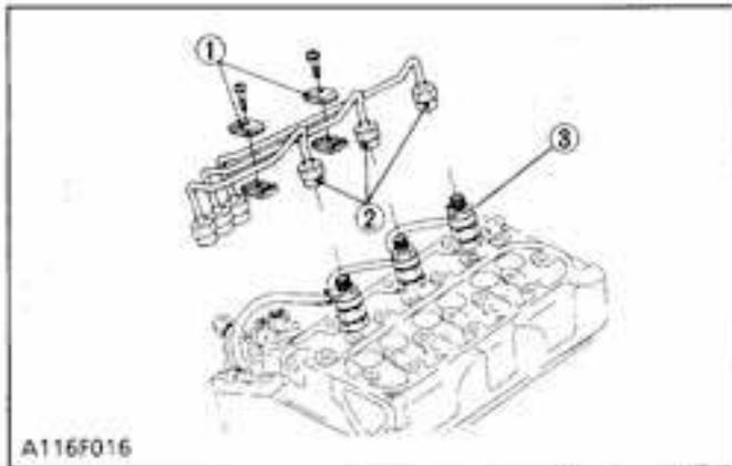
(1) Pipe Clamps (2) Injection Pipes (3) Nozzle Holder Assembly
