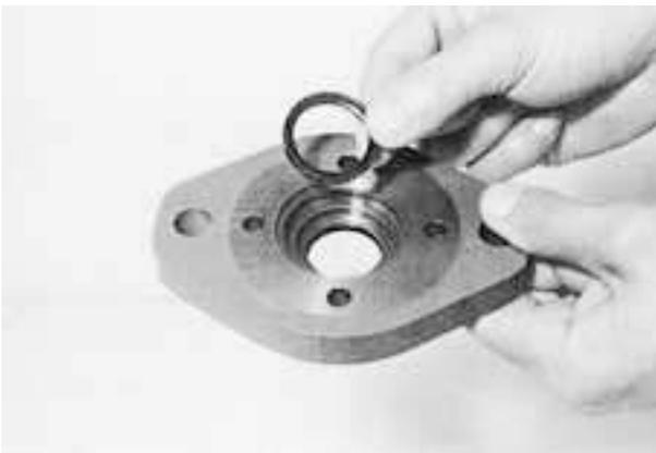
(5) Install oil seal in flange as shown in Fig.
