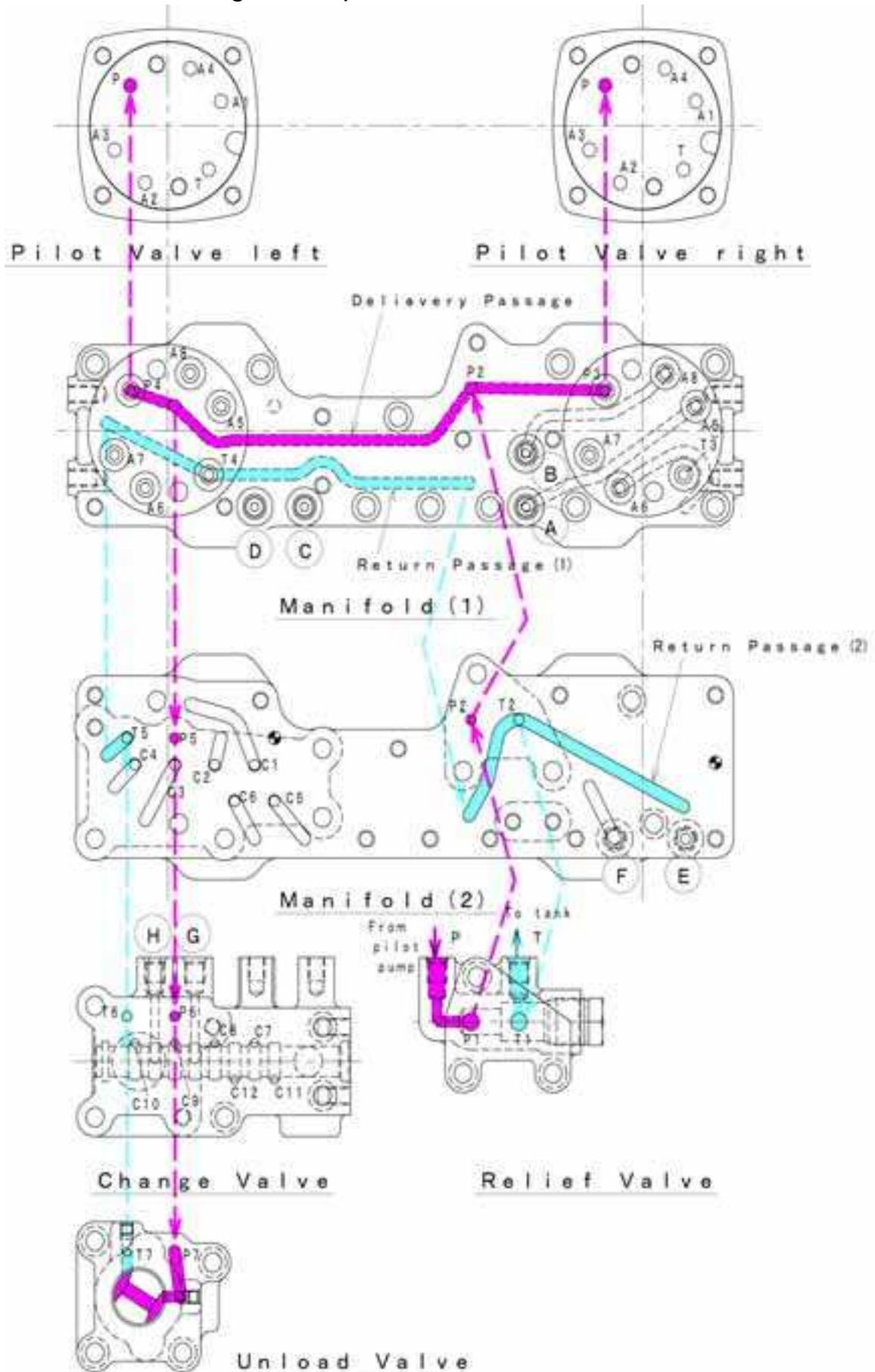
b. Flow of oil at the time when the control lever lock is at unlock position
