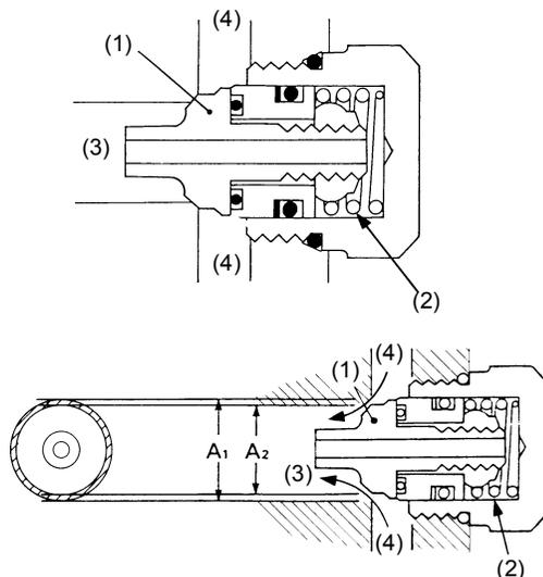
If the pressure (3) at the cylinder causes cavitation, the anti-void valve opens itself, feeding the oil from the tank and filling the space.
