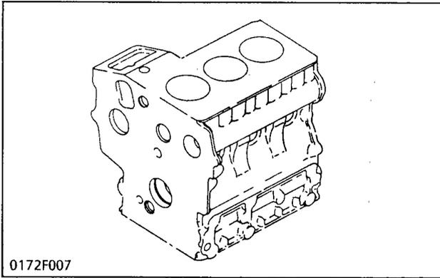
The engine has a high durability tunnel-type cylinder block in which the crank bearing component is a constructed body. Furthermore, liner less type, allow effective cooling, less distortion, and greater wear-resistance. The noise level is reduced to a minimum because each cylinder has its own chamber.
