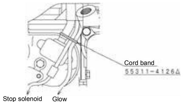
\* Clamp the wire harness to the engine breather's iron part.
