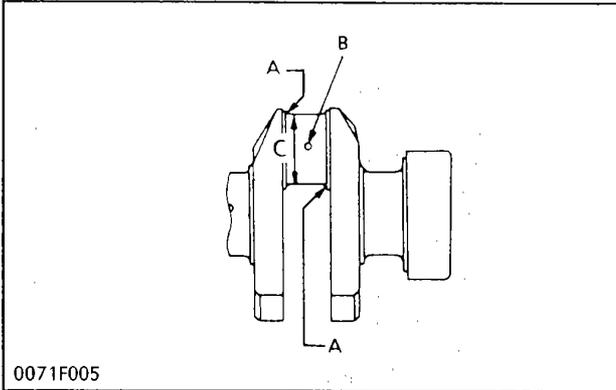
**Oil Clearance between Crank Pin and Crank Pin Bearing**
