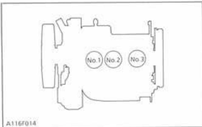
The cylinder numbers of 68 mm STROKE SERIES diesel engine are designated as shown in the figure. The sequence of cylinder numbers is given as No.1, No.2, No.3 starting from the gear case side.
