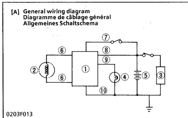
The regulator performs rectification and voltage regulation. The regulator converts AC into DC which flows through the power consuming circuits and the battery, and also charges the battery. If however, the battery voltage exceeds a certain level. The DC current is cut off from the charging circuit to prevent overcharging.
