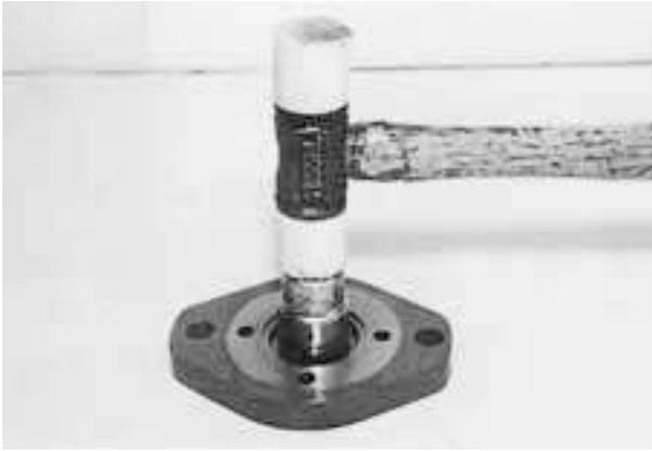
When press fit the dust seal and oil seal, use socket and tap in with hammer.
