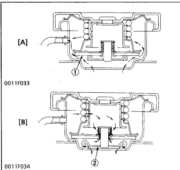
The radiator cap is for sustaining the internal pressure of the cooling system at the specified level 88 kPa (0.9 kgf/cm<sup>2</sup>, 13 psi) when the engine is in operation. The cap consists of a pressure valve (1) a vacuum valve (2), valve springs, gasket, etc.
