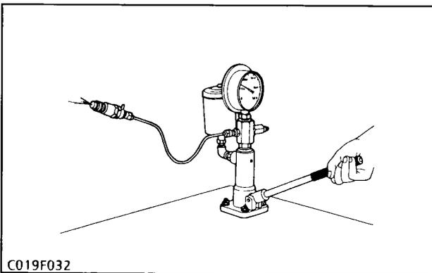
**Checking Nozzle Injection Pressure**
