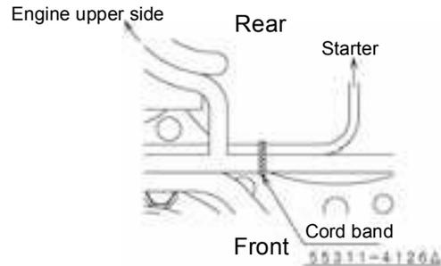
\* Securely clamp the wire harness (1) and the battery.
