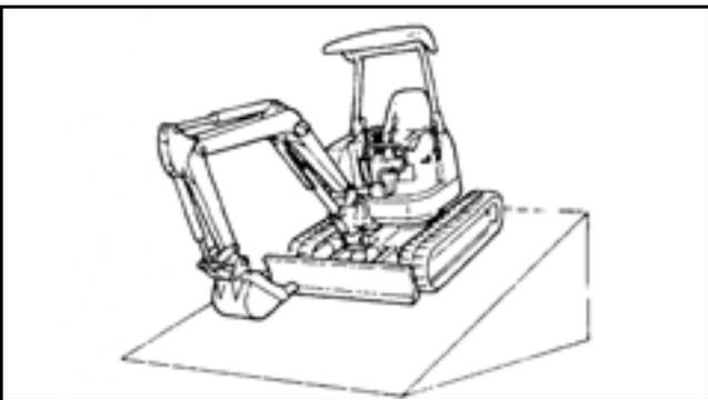
1. Park the machine on a 20deg. slope. Keep front at traveling position.
