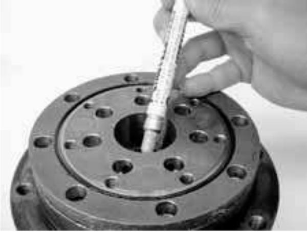
14) Mount the valve plate (17). Phase position can be aligned by matching with the wheel hole. Put a mark by felt pen to the same phase position as the position where the valve is marked.
