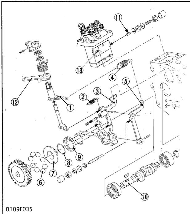
The governor controls the amount of the fuel to be fed in the entire speed range to prevent the engine from changing its speed according to the load.
