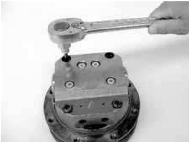
10) Fix the wheel and remove four M8 bolts (28) by which the end cover assembly is mounted.
