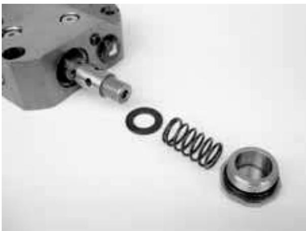
11) Remove the plug (V11), and then remove the spring (V9), washer (V13) and spool (V7).
