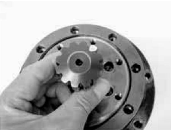
15) Put a mark to one of the teeth of the drive (20) and fit it in by matching to the mark of aforesaid hole side.
