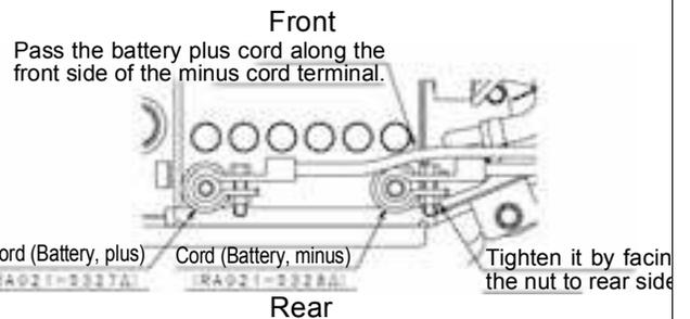
\* Tighten the cord (battery, minus) so that the nut comes to the rear side.
