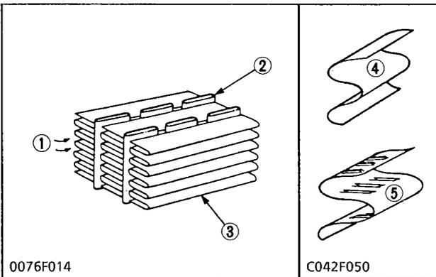
The radiator core consists of water carrying tubes and fins (3) at a right angle to the tubes (2). Heat of hot water in the tubes is radiated from the tube walls and fins. KUBOTA's engine uses corrugated fin type core which has a light weight and high heat transfer rate. Clogging is minimized by the louverless corrugated fins.
