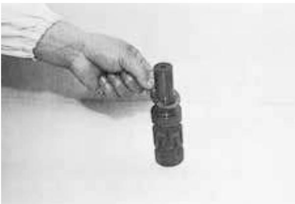
(10) Take out needle bearing from output shaft.
