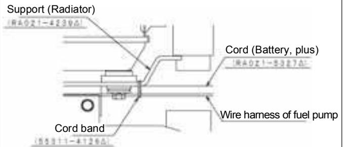
\* Clamp the battery plus cord and the wire harness of solenoid pump to the support (radiator).
