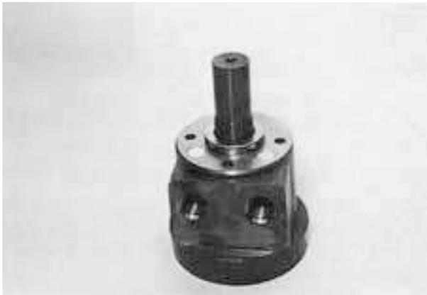
(3) Install output shaft in housing.
