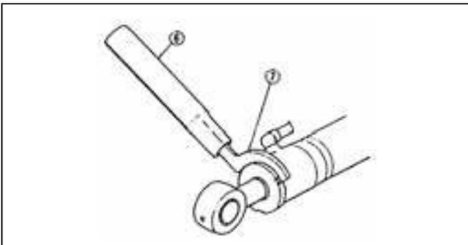
4. Loosen the cylinder head screw and detach the cylinder head.
