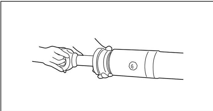
5. Draw out the piston rod together with the cylinder head.
