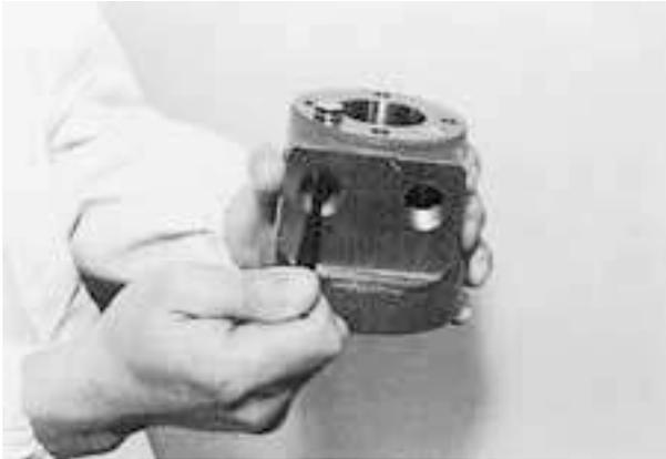
(17) Take out two plugs from housing. Inserting through port hole, push up the plugs. If not in need, never remove check plug.
