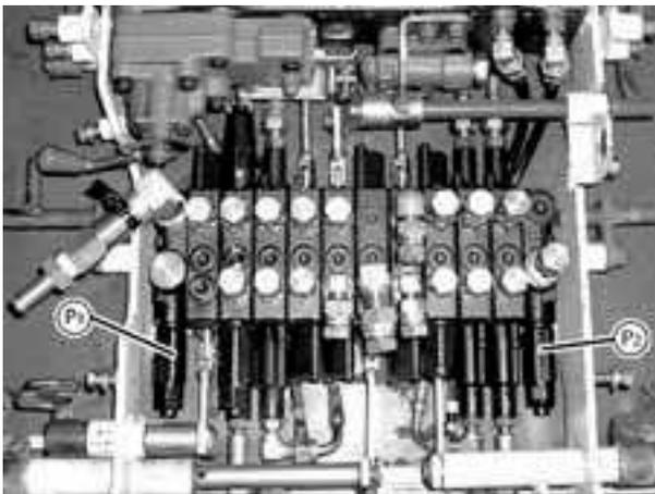
Arrangement of control valve section
