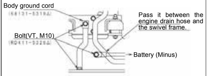
\* Pass the battery minus cord between the engine water drain hose and swivel.
