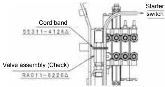
\* Pass the wire harness through the inside of the valve assembly (check) and clamp it securely.
