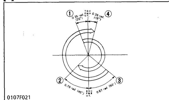
The timing for opening and closing the valve is extremely important to achieve effective air intake and sufficient gas exhaust.
