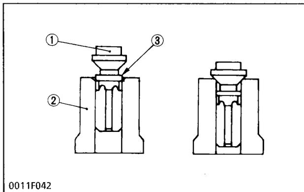
The delivery valve consists of the valve (1) and the Valve seat (2).
