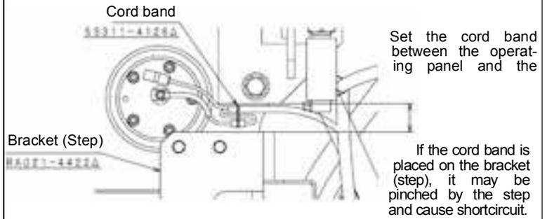
\* Insert the clamped wire harness between the operation panel and the bracket of step.
