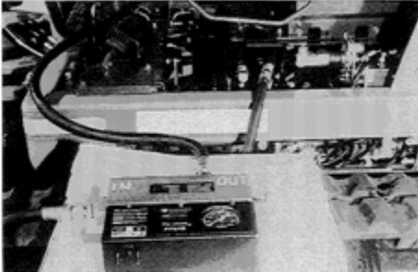
1. Connect the tester to the pump discharge side. Be careful not to connect the wrong pipes.
