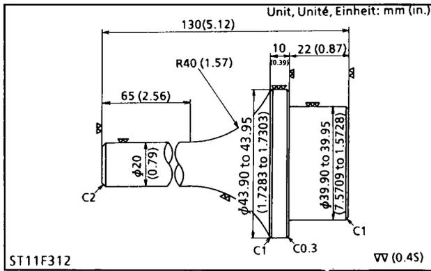
**Crankshaft Bearing 1 Replacing Tool**
