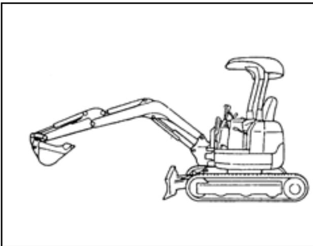
1. Position the boom, arm and bucket as shown at left. (with the bottom of the bucket about 1 m (33 ft) above from the ground.)
