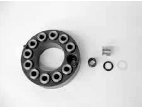
10) Insert the spring (15) in the valve and fit in the sleeve (22). If frictional force of sleeve's O-ring is large and the spring which is elongated up to the bottom will not return, push the sleeve slightly out of the valve hole.
