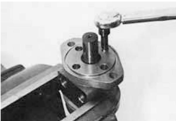
(10) Clamp at housing with vise and tighten 4 bolts. (Tightening torque 25.5 ~ 31.4N·m (2.6 ~ 3.2kg·m))
