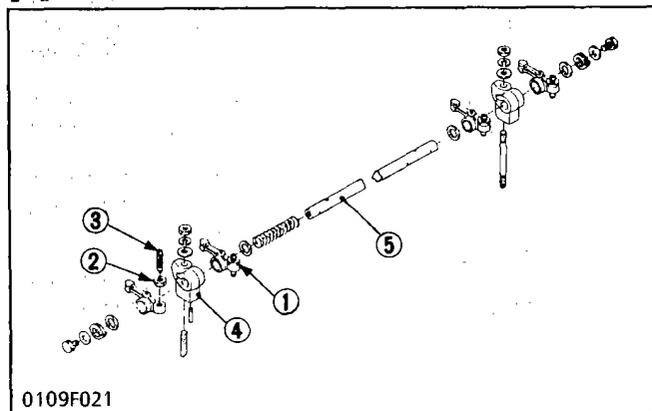
The rocker arm assembly includes the rocker arms (1), rocker arm brackets (4) and rocker arm shaft (5) and converts the reciprocating movement of the push rods to an open/close movement of the inlet and exhaust valves.
