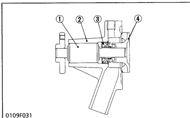
The water pump is driven by the crankshaft via a V-belt. Water cooled in the radiator is sucked into the water pump from its lower portion and is sent from the center of the water pump impeller (4) radially outward into the water jacket in the crankcase.
