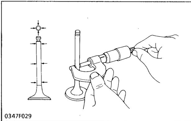
**Clearance between Valve Stem and Valve Guide**
