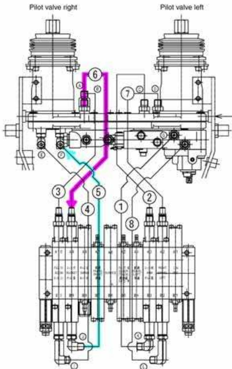
d. Flow of oil in bucket dumping operation
