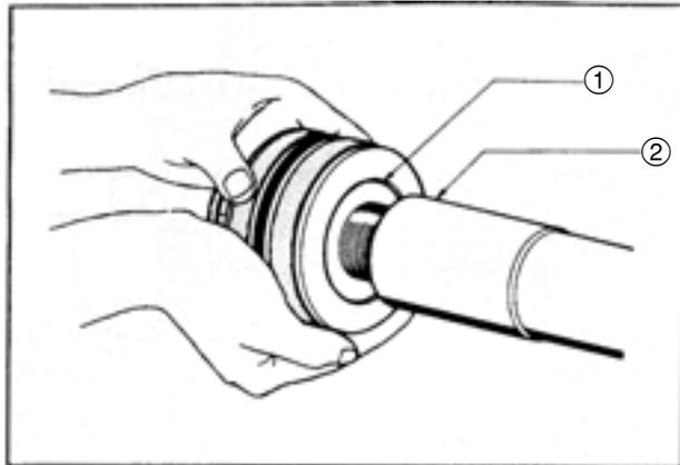
7. Draw out the piston and remove the shim
