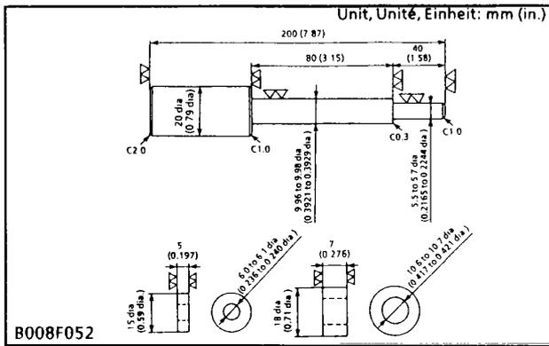
**Valve Guide Replacing Tool**
