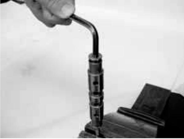
12) Remove the plug (V12) which is fitted to the spool (V7), and remove the spring (V10) and Counter-balance poppet (V8).
