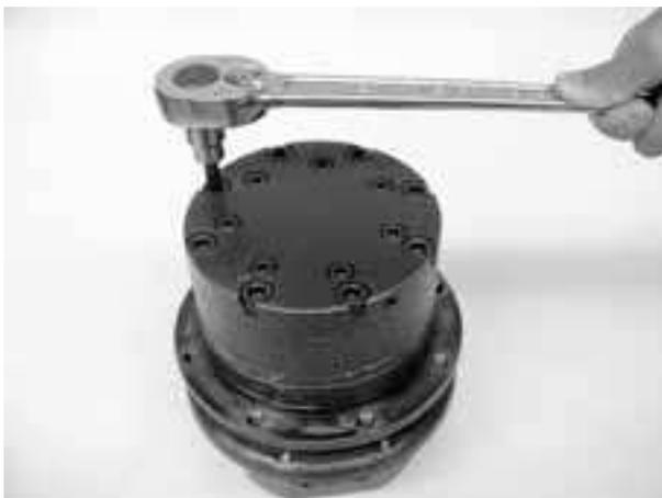
19) Tighten eight M10 bolts (24) and seven M8 bolts.
