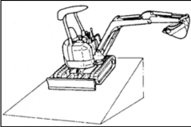
1. Locate the machine on the 15 deg. slope.
