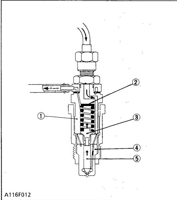
This nozzle is throttle-type. The needle valve (5) is pushed against the nozzle body (4) by the nozzle spring via the push rod (3). Fuel pressurized by the injection pump pushes the needle valve up and then is injected into the sub-combustion chamber.
