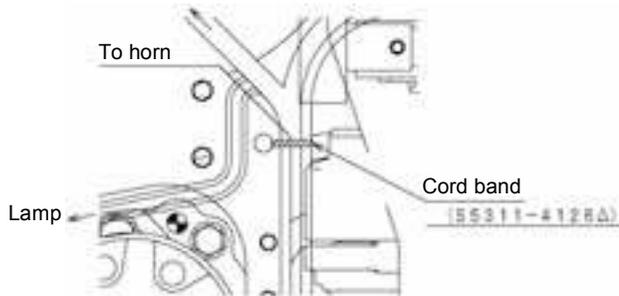
\* Clamp the battery plus cord and the wire harness (1) to the swivel frame.
