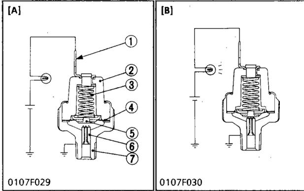
The oil pressure switch is mounted on the cylinder block and is led to the lubricating oil passage. When the oil pressure falls below the specified value, the oil pressure warning lamp lights.
