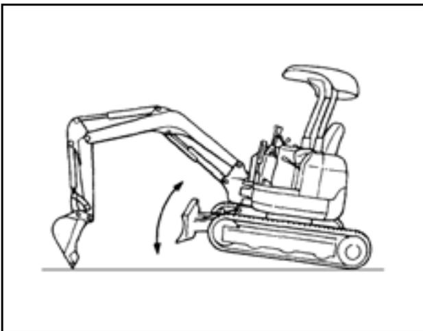
1. Place the bucket on the ground. Position the machine as shown at left for the dozer to make a full stroke.
