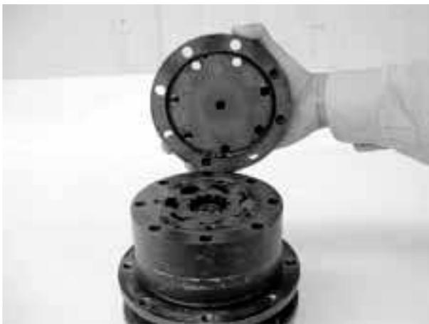
18) Fit the O-ring (26) to the geroller cover (18) and mount the motor.
