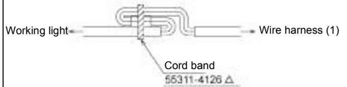
\* Clamp the wire harness of the working light securely.
