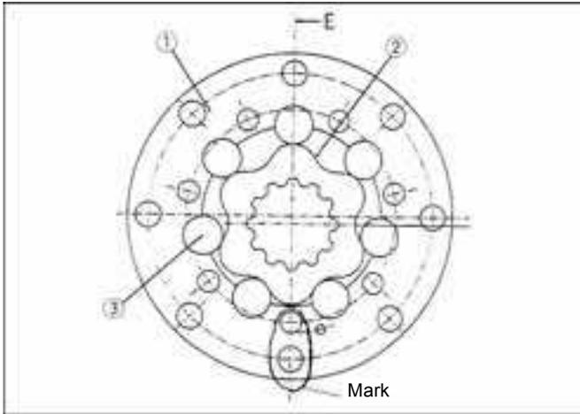
17) Clamp and fix the end cover assembly (27) and turn the wheel and valve plate to align it with the bolt holes of the geroller. (There is only one phase position to be able to match all the bolt holes.)
