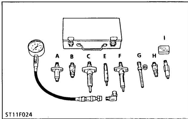
**Diesel Engine Compression Tester**
