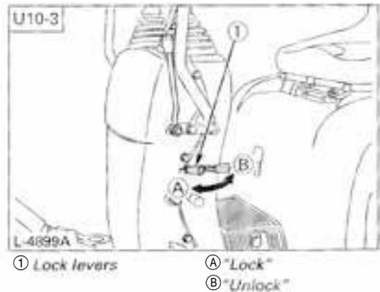
b. Control lever lock being at unlock position
