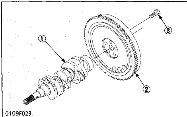
The flywheel stores the rotating force in the combustion stroke as inertial energy, reduces crankshaft rotating speed fluctuation and maintains the smooth rotating conditions.
