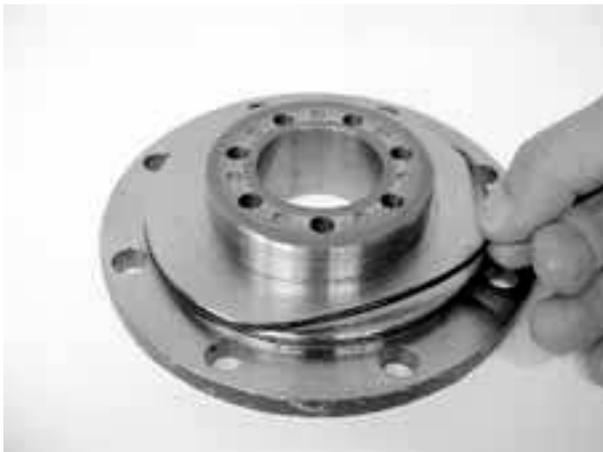
13) Fit the O-ring (20) to the valve plate (17).
