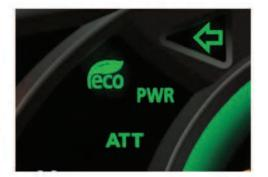
Select Eco mode to reduce fuel consumption, up to 15%, by limiting the engine rpm. This mode is exchanging high traction force for handling material in the yard or load and carry functions for fuel savings.
