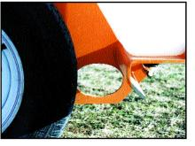
Large, well placed tie down points allow quick and efficient tie down when hauling and prevents damage due to improperly placed restraints.
