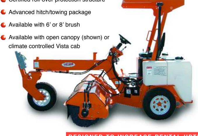
Proven and accepted as #1 leader in the rental sweeping industry, the Lay-Mor Model 6HC/8HC is operator friendly and is easily transported from job to job. There is no need to raise the front wheel off the ground for towing purposes and the tongue can pivot right or left and up and down for faster and easier hook-up. More easily accessible maintenance allows for servicing the unit quicker and simpler than competitive products.
