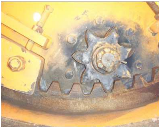
Figure 7-18. Turntable Pinion Gear
