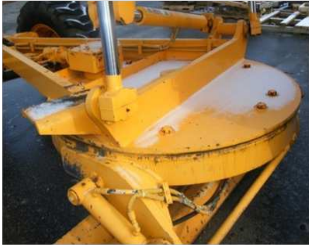
Figure 7-17 Moldboard Turntable Assembly
