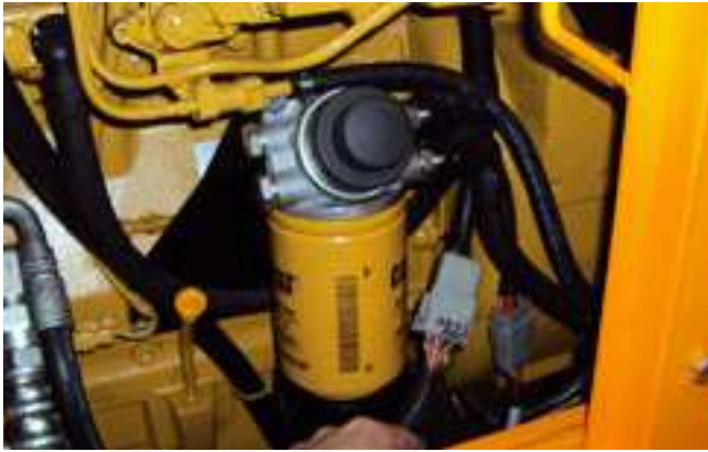
Figure 7-2. Location of Fuel Drain Valve
