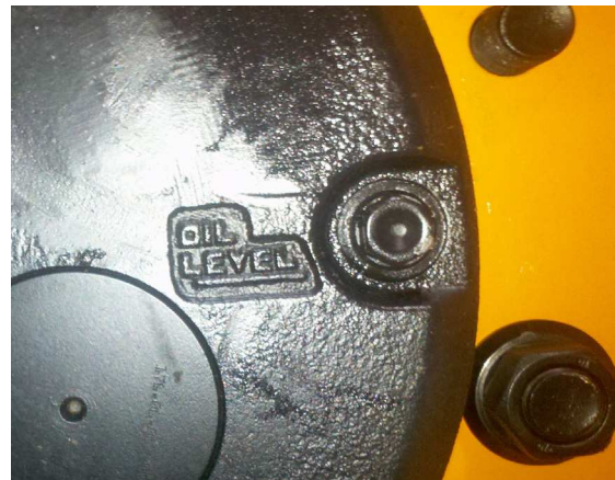
Figure 7-7. Hub Oil Check Bolt
