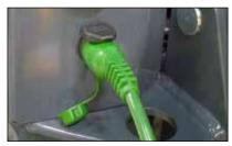
Engine heater for cold temperatures
