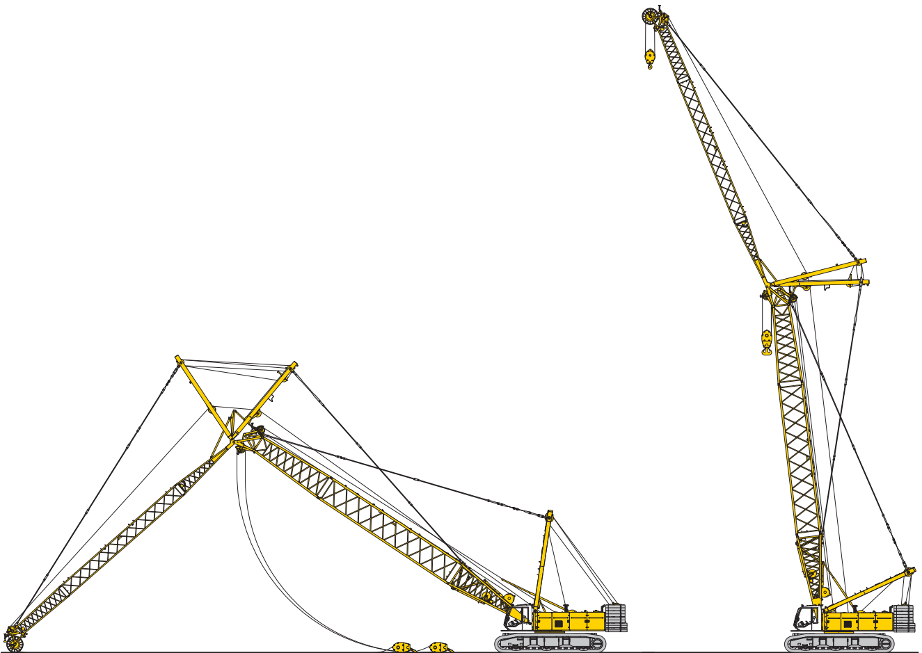
Erecting of main boom and luffing jib
