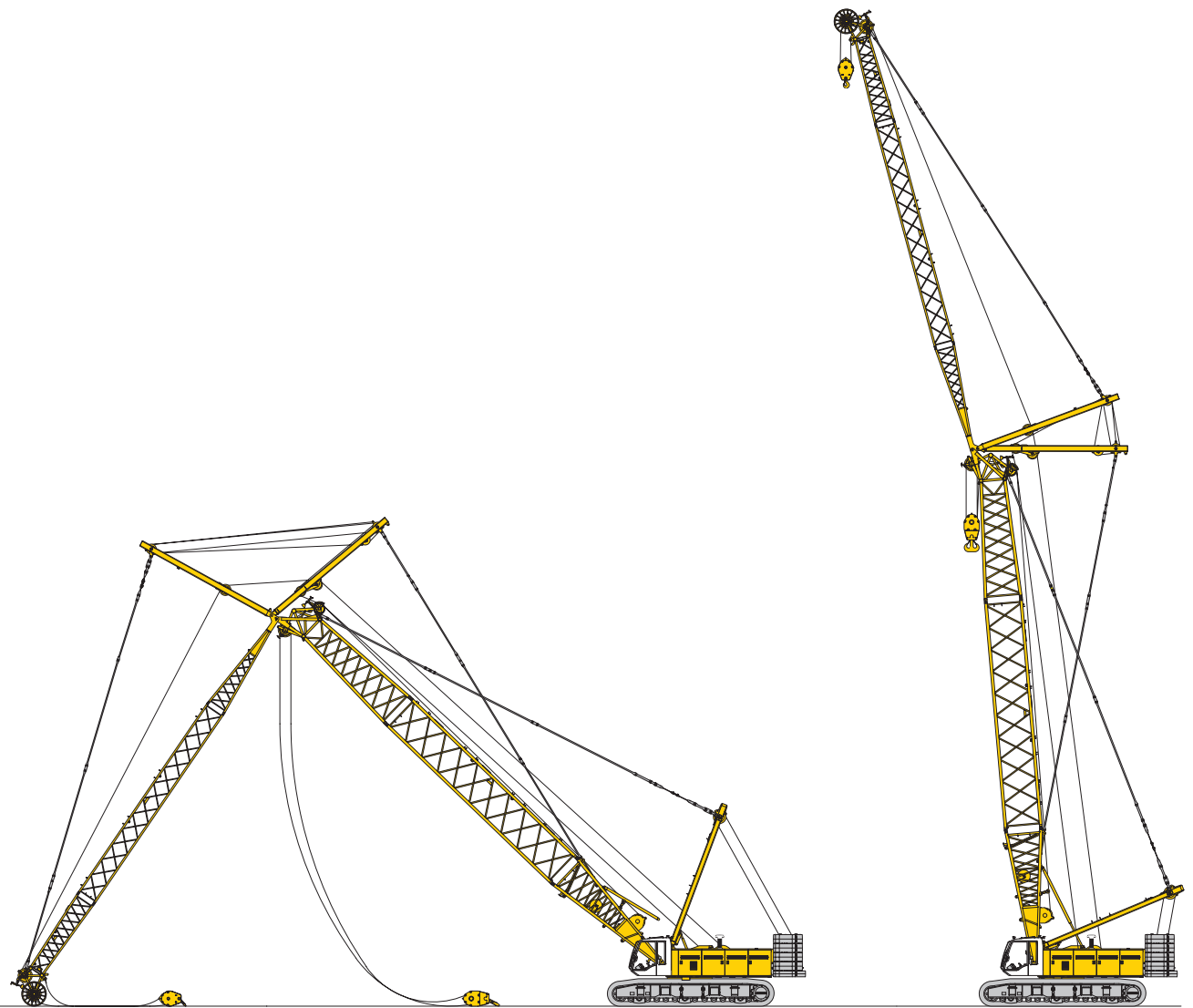
Erecting of main boom and luffing jib
