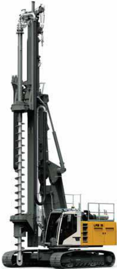
LRB 16 — Effective length – 18.4 m with auger cleaner
