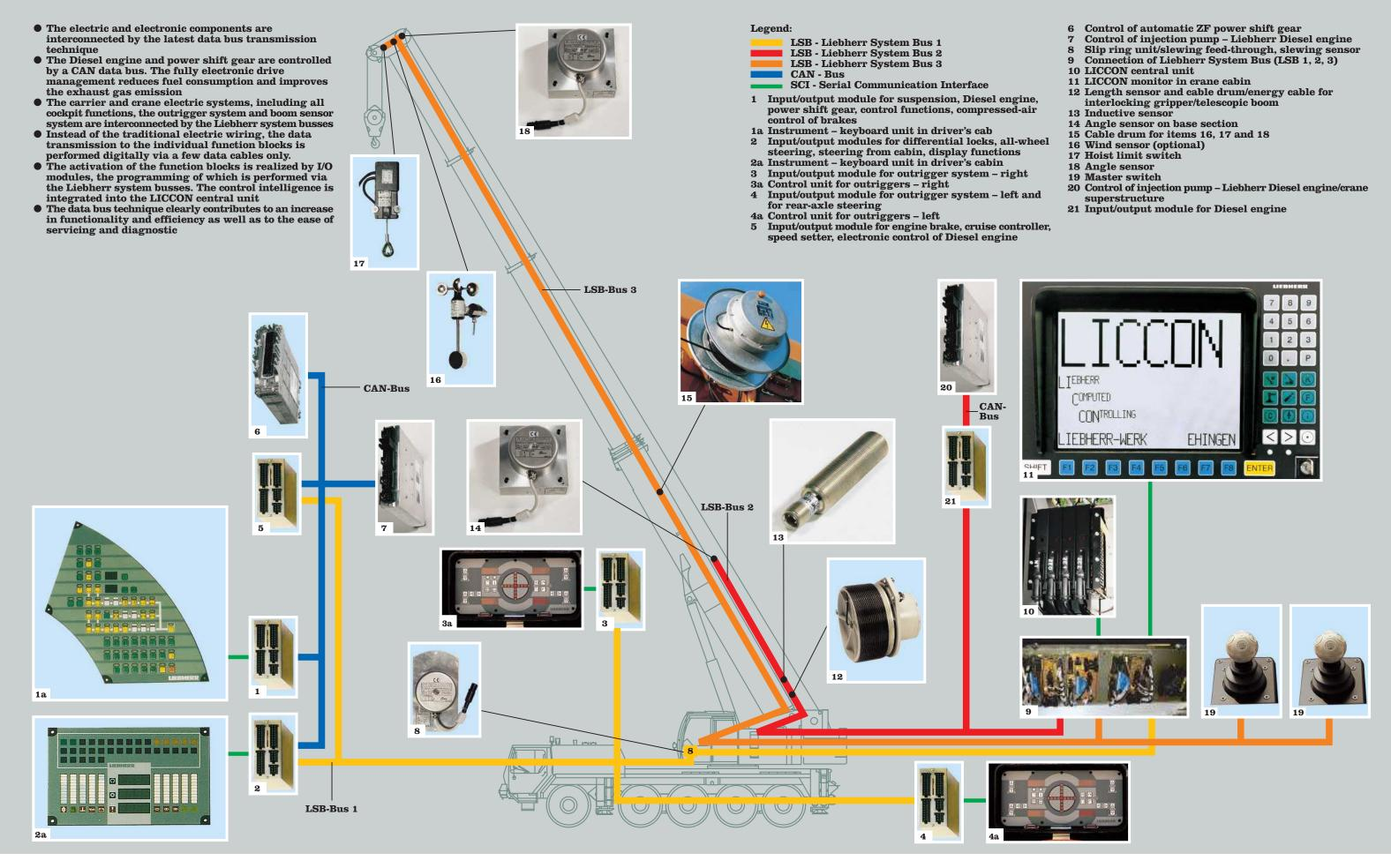
Data bus technique revolutionizes crane electric system.
