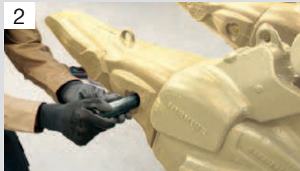
2 Remove the securing pin from the mounting.
