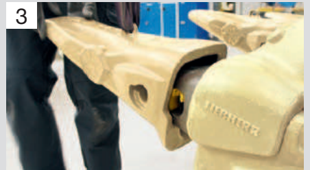
3 Draw the worn tooth from the tooth adapter.
