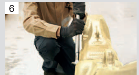
6 Lock the securing pin with the locking spanner.
