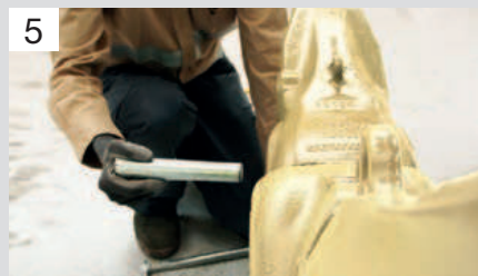
5 Slide the securing pin into the mounting.
