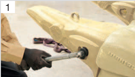
1 Unlock the securing pin with the locking spanner.
