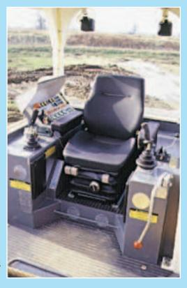
The pipe layer can also be equipped both with a canopy and a fully enclosed operator's cab.
