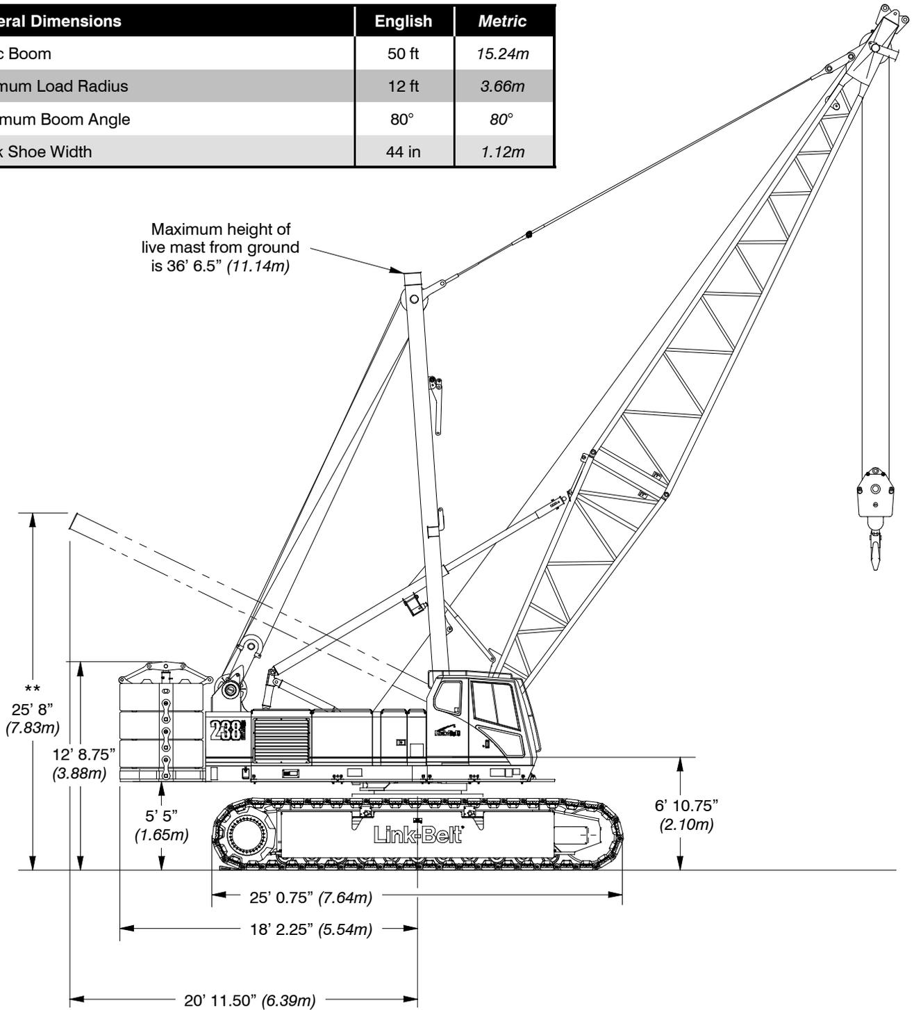
Note: \*\* @ Maximum boom angle (80°) with maximum boom [260 ft (79.25m)], maximum rotation radius occurs.
