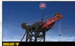
With a maximum of capacity of 25 tons, the newly designed auxiliary tip extensions provides excellent capacities and load line separation during 2 load line operations.
