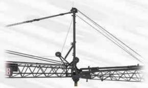
The rear post is supported in the vertical position by the back stop tubes during assembly.
