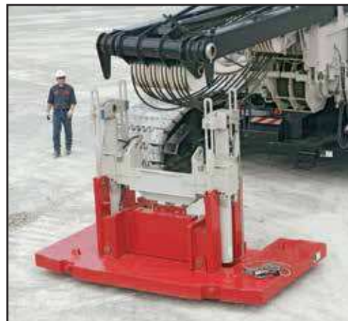
Counterweight removal mechanism detached
