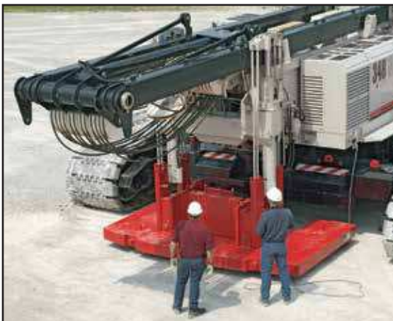
Counterweight removal mechanism self-removes for even lower main load transport weight where required.
