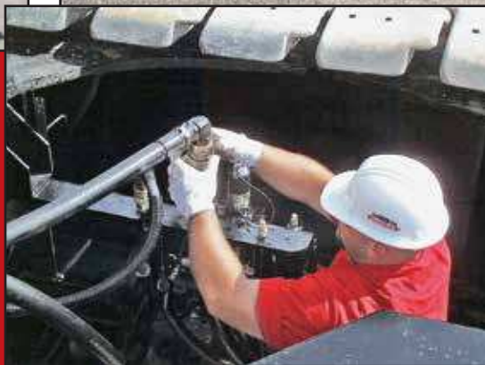
Crawler quick disconnects can attach in minutes — no tools required
