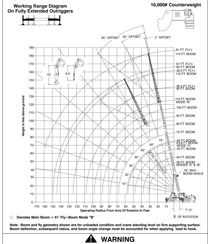
Do Not Lower The Boom Below The Minimum Boom Angle For No Load As Shown In The Lift Charts For The Boom Lengths Given. Loss Of Stability Will Occur Causing A Tipping Condition. CONSTRUCTION EQUIPMENT
