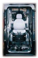
**Operator's Control Station** Offers superior visibility and more! The operator's control station is designed with the operator in mind, and is mounted to the frame on six fluid filled mountings for minimal vibration. Features include a wide opening door, a cloth upholstered suspension seat with integral headrest and armrests, heater with 3-speed fan, AM/FM radio, cigarette lighter, pop-up skylight window, oscillating fan, and intermittent windshield wiper with washer.
