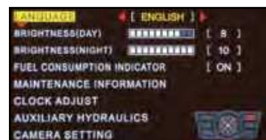
From the Computer Menu, you can change the monitor language, program service reminders and change auxiliary settings for flow and pressure to name a few.
