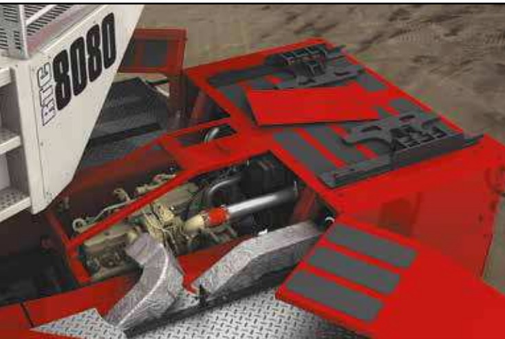
Swing-out doors provide exceptional access to engine components.
