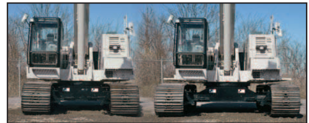
32" grouser track shoes form a wide gauge of 11' 2" (3.40 m) when extended, and 8' 9" (2.66 m) when retracted with two position house lock.
