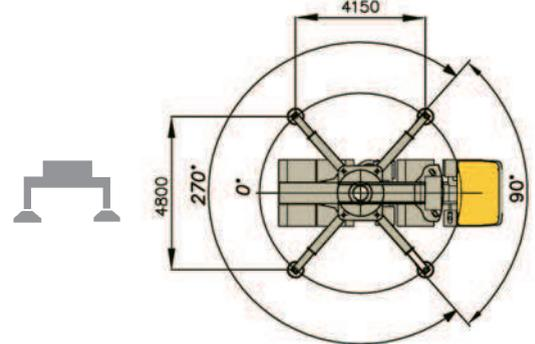
The lifting capacities indicated are in accordance with DIN 15019 part 2 and ISO 4305.
