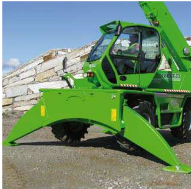
◀ Folding stabilisers on Roto 400 series models.
