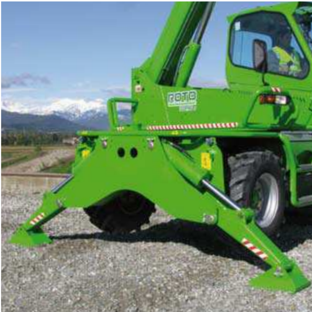
◀ Stabilisers with independent extension and jacking on Roto MCSS. Additional load-spreading plates can be used in softer ground.
