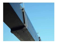
**Easy Glide boom** wear pads Easy Glide boom wear pads reduce the conditions that cause boom chatter and vibration. The net result is smoother crane operation.
