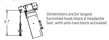
\*Drawing is to show the physical reach of the machine. Always refer to load chart to see what portions of this range are structurally and stability limited.
