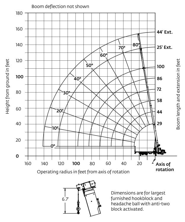
\*Drawing is to show the physical reach of the machine. Always refer to load chart to see what portions of this range are structurally and stability limited.
