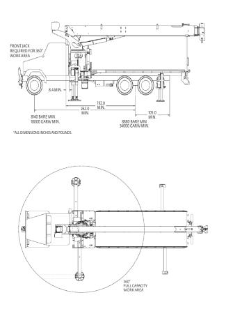
Note: Chassis will require extended front frame rails for SFO addition.
