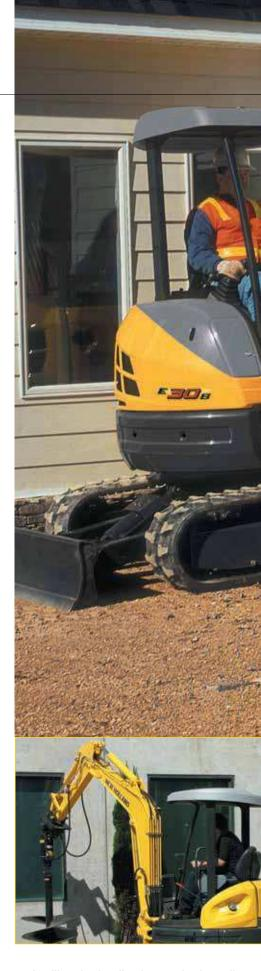
Auxiliary hydraulics is standard on all models. Run hammers using the single acting circuit or use the selector valve to give dual acting flow to run augers and nibblers.
