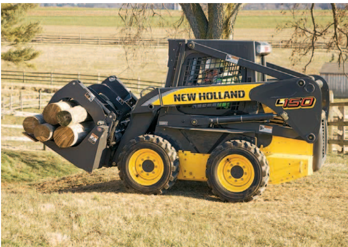
L150 is shown with the grapple attachment.
