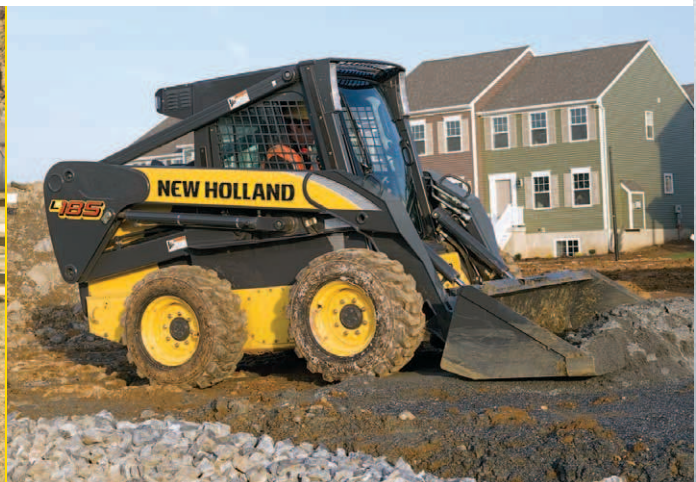
L185 is shown with the bucket attachment.
