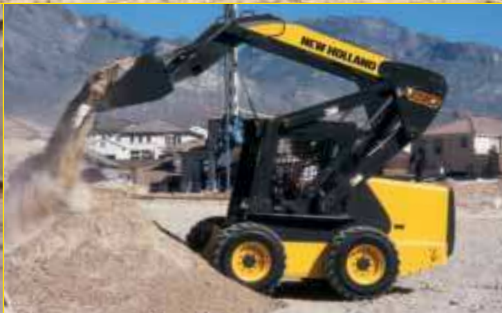
An exceptional 45° dump angle and 36° rollback angle help boost your productivity.
