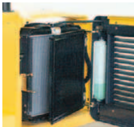
A new higher cooling capacity radiator improves engine cooling during extended operation and in high temperatures.
