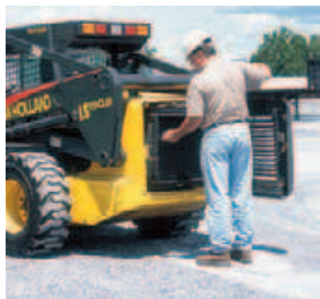
It's simple to reach all major service points—even with the boom down.
