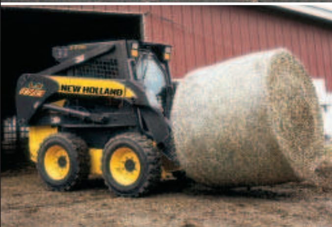
The long LS wheelbase and low center of gravity provide added stability on uneven terrain.
