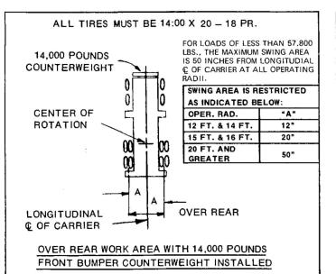
MAIN HOIST DRUM RATED LOADS FOR SEVEN-EIGHTHS INCH DIA. P&H TYPE 4 WIRE ROPE (6 x 25 WITH FILLER WIRE, PRE-FORMED IMPROVED PLOW STEEL WIRE ROPE, 7 x 7 I.W.R.C.)
