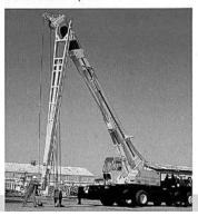
extended when necessary. For storage, the extended jib is twisted so that its sides face up and down, and then turned upward to be held beside the boom. This storage arrangement assures the driver safe travelling with a wider view. Since the jib is turned downward for extension, the space required for setting can be minimal. Setting is easy even in confined areas.
