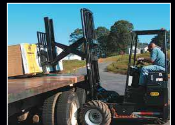
Lift capacity is 5000 lbs. at 24" load center
