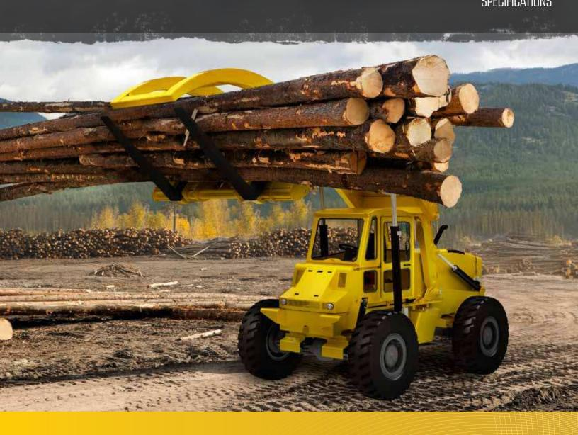
Equipped with a special wood baler, the newly redesigned Cary-Lift™ 154 is more productive, easier to service and more cost-effective than ever before. The 154 offers wider lift arms and front balers for enhanced load stability, along with the Pettibone® patented lift arm design for full front visibility and safer operation in wood yards. Featuring an IQAN® controlled electrohydraulic system, the 154 is built for optimal efficiency.
