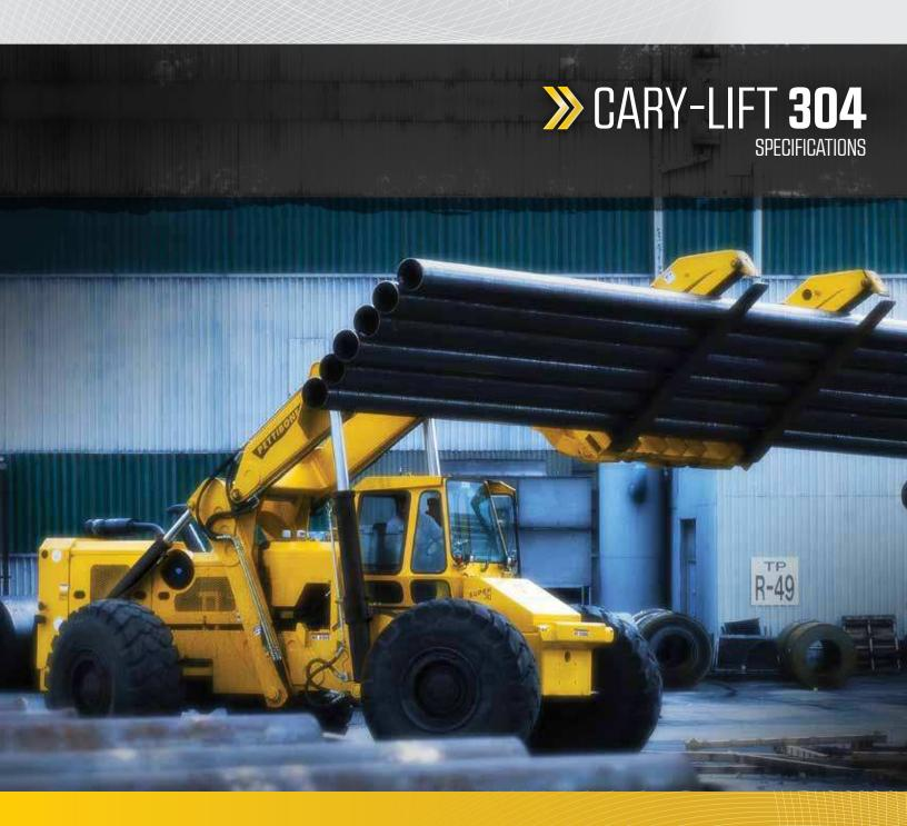
Ruggedly built to perform for the long haul, the Cary-Lift 304 offers a number of engineering advantages, including an overhead lift arm design that provides maximum visibility when lifting or moving loads. Featuring components like heavy-duty 4-wheel drive axles and a load-sensing hydraulic system, the 304 is stronger and smarter, allowing it to tackle the most demanding material handling jobs time and again.
