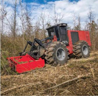
The heart of the 2864C hydraulic system is the new PowerDirect Plus system, which goes beyond load-sensing to efficiently distribute power to increase the capability of each system and maximize productivity.
