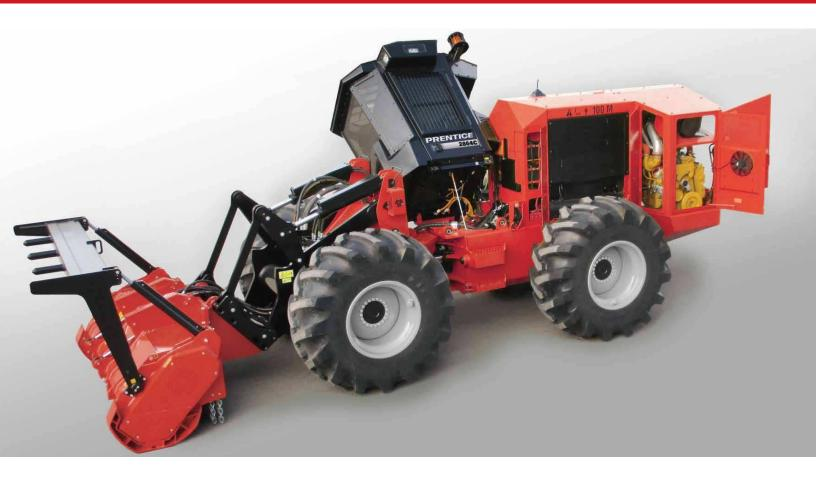
Daily service points are in easy reach on the 2864C. Add hydraulic oil with the electric pump and refuel with your boots on solid ground. The tilting cab and hinged panels give you access to even more.
