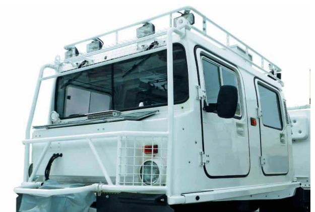
Body, glass and headlight guards allow the vehicle to travel through forest areas
