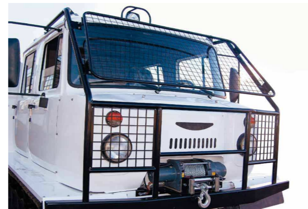
Body, glass and headlight guards allow the vehicle to travel through challenging forest areas
