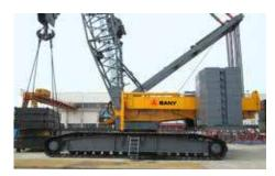
Counterbalance Equalization) System automatically adjusts the counterweight position to the boom angle. Employing an upperworks tray, hanging brackets and upper sideblocks, the ACE System reduces overall crane weight and allows the SCC8500 to be transported like
