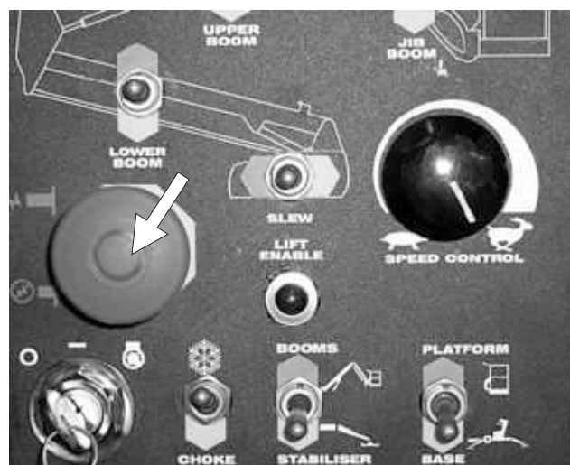
Figure 8.1 - Ground Control Box Emergency Stop Switch Location.
