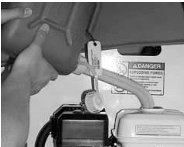
Correct Method to Fill MHP13/35 / MHP15/44 Mark II Fuel Tank
