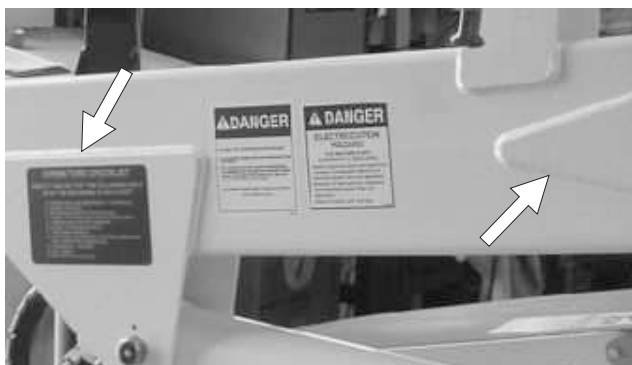
Figures 7.17 - Boom Welds
