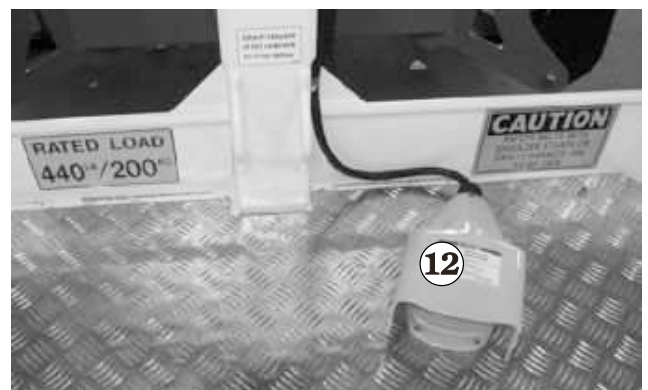
Upper Controls Foot Switch
