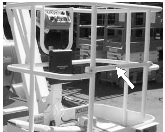
Figure 7.19 - Platform Gravity Gate
