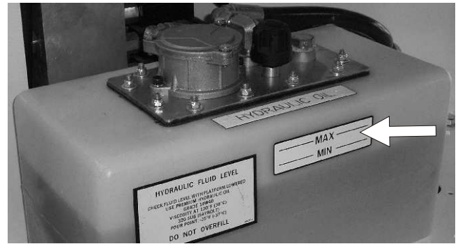
Figure 7.9 - Hydraulic Oil Level
