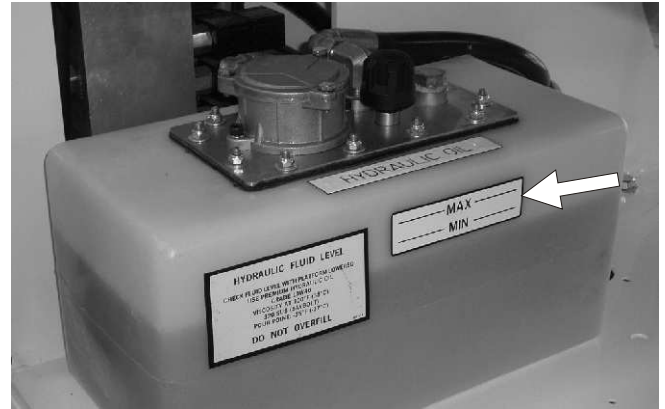
Figure 4.3 - Hydraulic Oil Level
