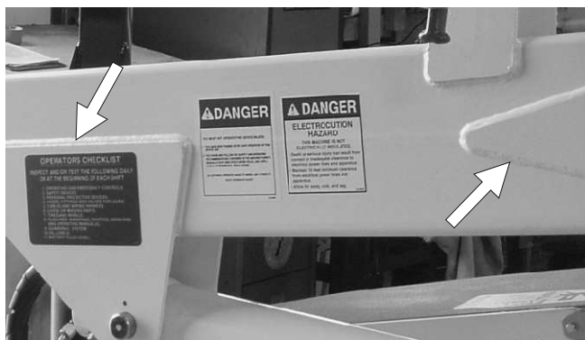
Figures 7.18 - Boom Welds
