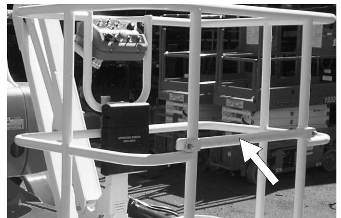
Figure 7.20 - Platform Gravity Gate
