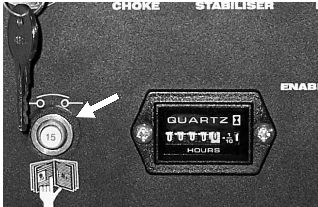
Figure 5.2 - Main Circuit Breaker
