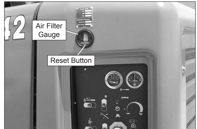
Figure 5.3 – Air Filter Gauge
