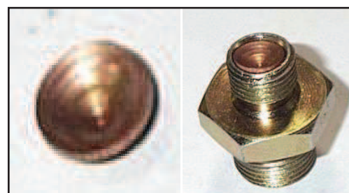
Figure 3-14: Copper restrictor fitted loose in the hose adaptor. Hose end requires more torque to prevent oil leak when securing hose.
