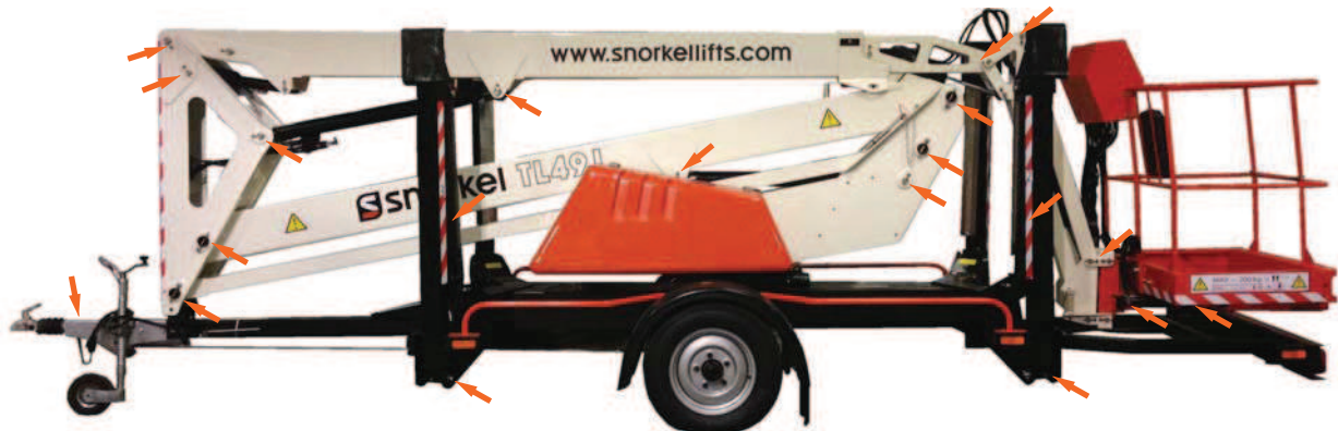
Figure 3-35: General grease point locations.
