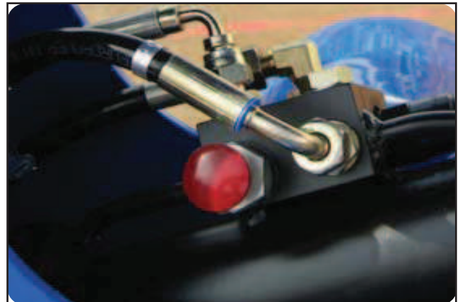
Figure 3-29: Emergency lowering valve.
