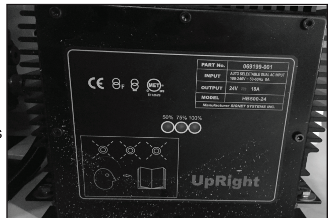
Figure 3-23: The charger (black box) shown has a 110 V plug. To operate on 240 V, replace plug.
