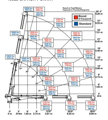
Weight of load handling devices are part of the load lifted and must be deducted from the capacity.
