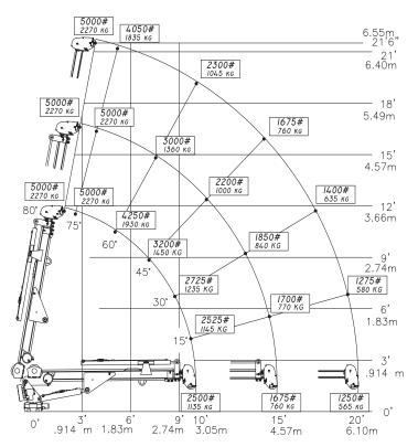
Weight of load handling devices are part of the load lifted and must be deducted from the capacity.
